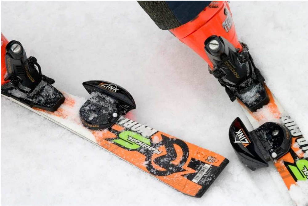
Figure 2. vLink shuttles mounted on skis. Set to measure inside edge of outside ski. 104x69mm (240 x 240 DPI)
