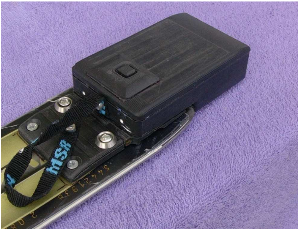
Figure 5. Early vLink prototype with sensors mounted on the tail of a ski. 125x96mm (200 x 200 DPI)
