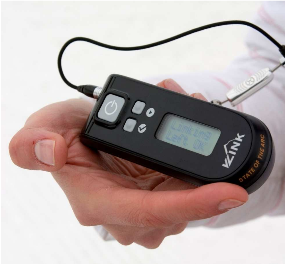
Figure 3. vLink remote with ear buds for real-time audible feedback. 104x96mm (240 x 240 DPI)
